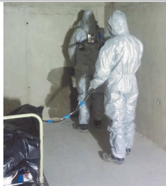
Figure 2: Workers in Romania and Poland performing various works involving materials with MNMs, with simultaneous measurement of the NP concentrations in air.
