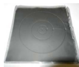
Figure 3. Electrode fabricated using the dynamic spray-gun method and composed of mixtures of graphene/graphite and CNTs
